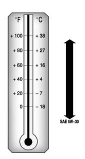
Cold Temperature Operation: In an area of extreme cold, where the temperature falls below -29°C (-20°F), an SAE 0W-30 oil should be used. An oil of this viscosity grade will provide easier cold starting for the engine at extremely low temperatures. When selecting an oil of the appropriate viscosity grade, be sure to always select an oil that meets the required specification, dexos™. See "Specification" for more information.
